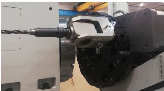
Moduli assiali e radiali per torretta a disco Axial and radial live tool modules for disk turrets
